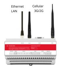
technical support. The interface automatically chooses the best available technology for the connection, 3G if possible and 2G if not. Different parameters are required: an APN with an optional username and password and a PIN code. The platform automatically recognizes the name of the network operator, the quality of the cellular signal, the technology used, the IMEI and IMSI number.
