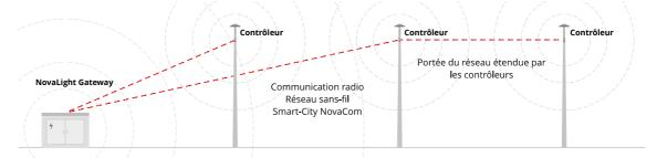
A communication between controllers usually takes place in a few tens of milliseconds. The depth of the network - i.e. the number of intermediate controllers allowing the network to be extended - is limited to 15 hops, which means that a single NovaLight Gateway could cover more than 2.5km with its network for a longitudinal route thanks to the relays.
